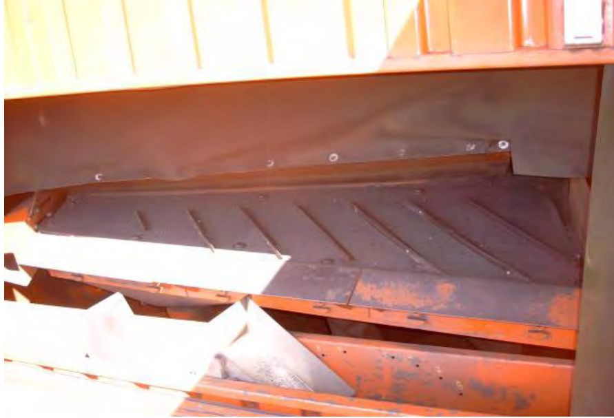
Figure 4. Deck (1 m 2 ) of the FGX air table.
