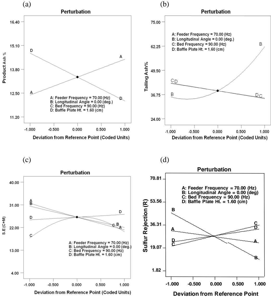
Figure 9: Perturbation plots for various process responses: (a) product ash content, (b) tailings ash content, (c) separation efficiency, and (d) sulfur rejection.
