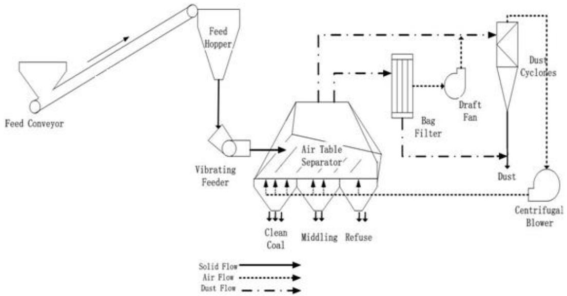
Figure 4: A schematic diagram of the FGX-1 Dry Separator test unit.
