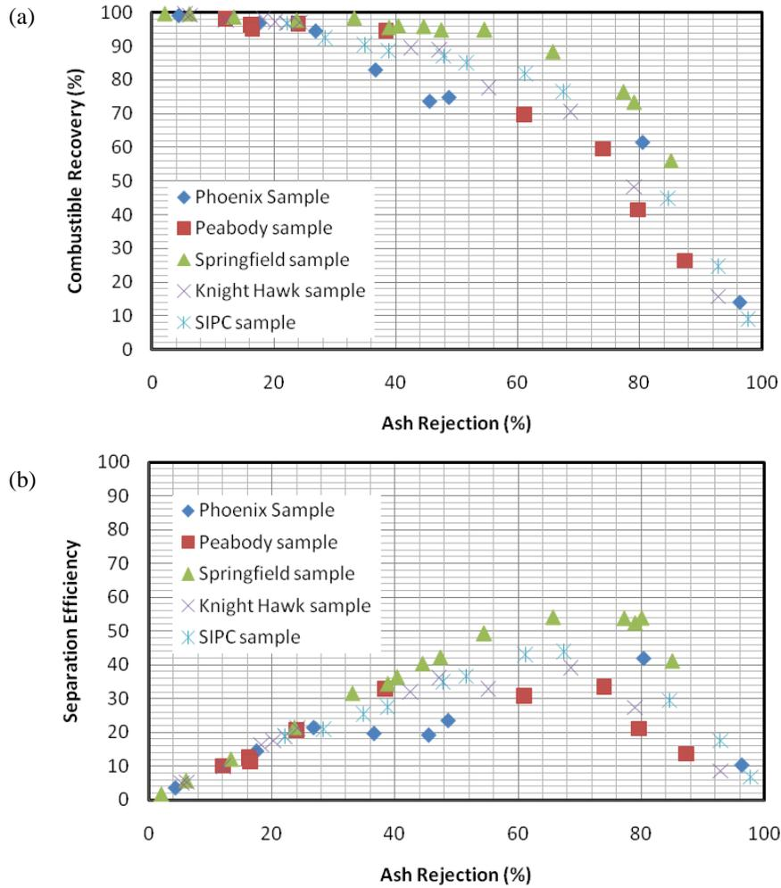
Figure 11: Model FGX-1 Dry Separator performance – ash rejection versus (a) combustible recovery and (b) separation efficiency.
