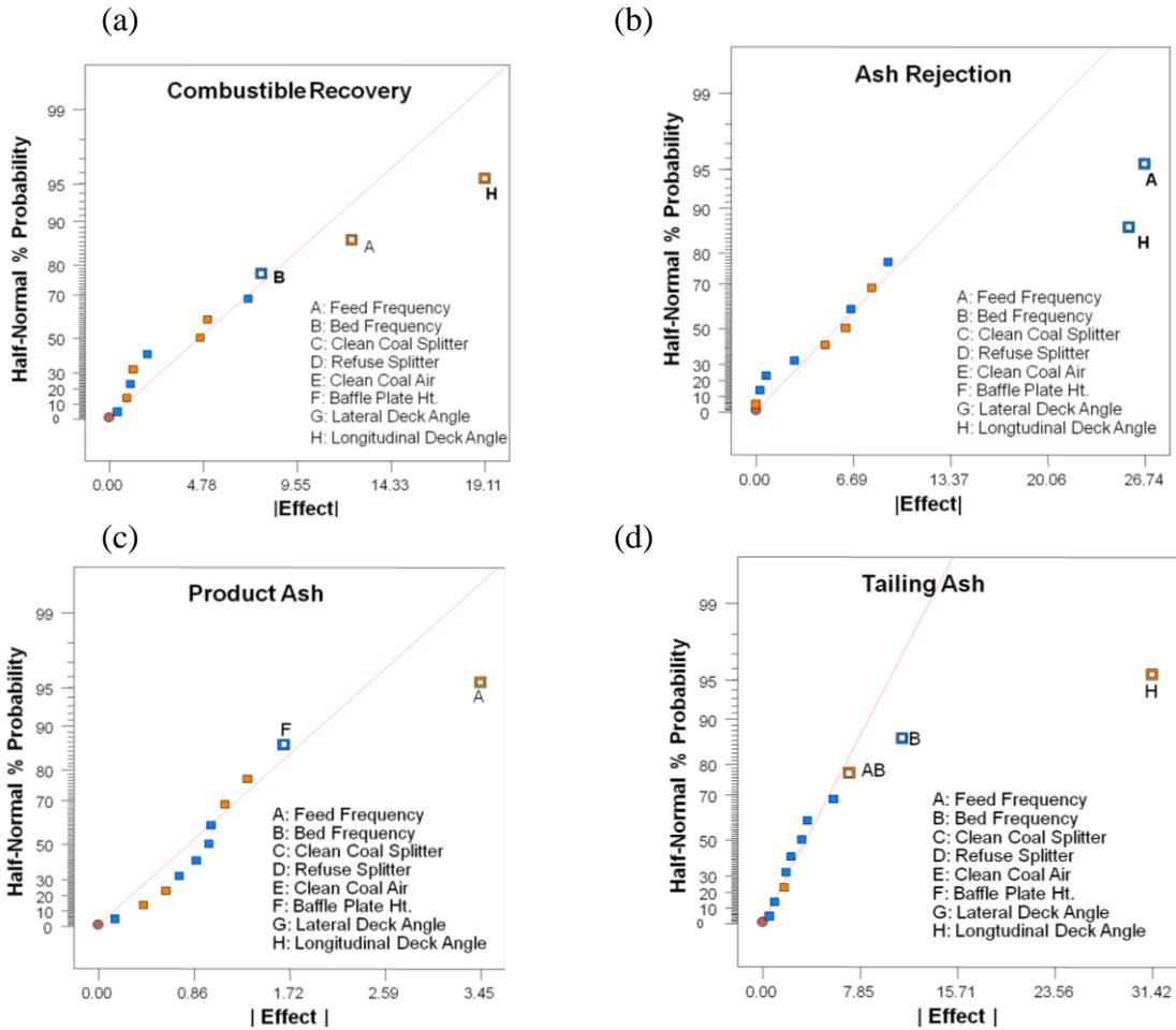
Figure 8: Half-normal probability plots generated from the Plackett and Burman experimental program identifying critical process parameters for the FGX Dry Separator.
