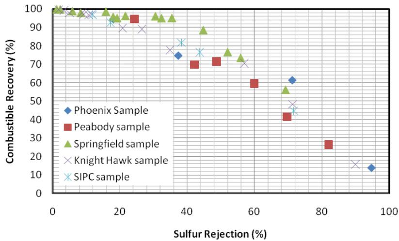
Figure 12: Model FGX-1 Dry Separator performance – sulfur rejection versus combustible recovery.
