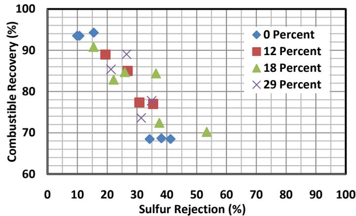
Figure 14: FGX Dry Separator sulfur cleaning performance with varying proportions of coal fines (-4 mesh) in the feed.
