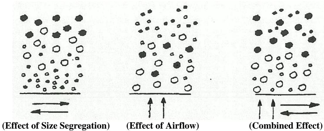
Figure 2: Stratification of feed material on the separating deck under combined effects of vibration and upward air pressure. Empty particles represent heavier solids (refuse) and solid particles represent lighter solids (clean coal) (Lu et al., 2003).
