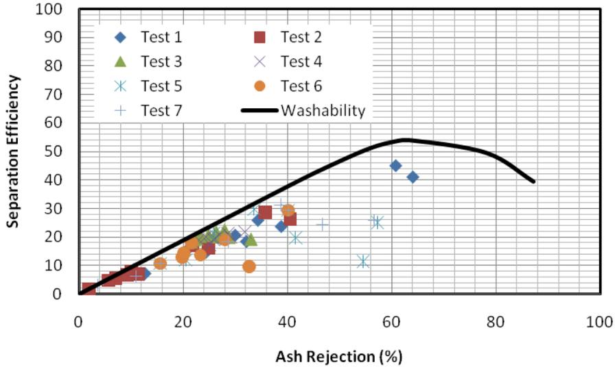
Figure 6: Ash cleaning performances for seven series of exploratory tests conducted with the Knight Hawk Coal sample. Test # represents Test Series # in Table 3.
