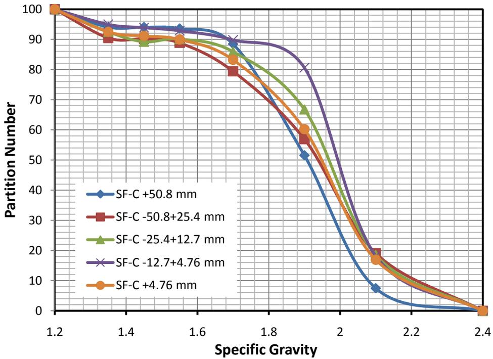
Figure 15: (a) Apparent and (b) corrected partition data for the Springfield Coal sample and for different size fractions of the same.
