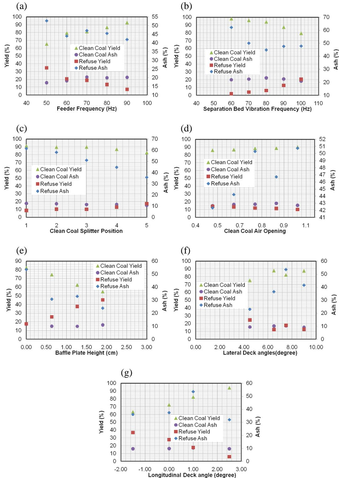
Figure 7: Preliminary investigation of FGX Dry Separator parametric effects during the exploratory test program.
