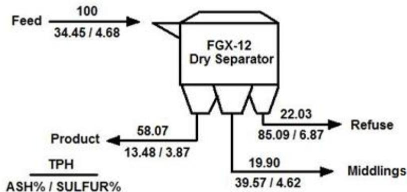
Figure 17: Schematic of proposed Model FGX-12 Dry Separator plant for processing easy-to-clean Illinois coal.
