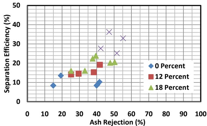
Figure 13: FGX Dry Separator ash cleaning performance with varying proportions of coal fines (-4 mesh) in the feed.
