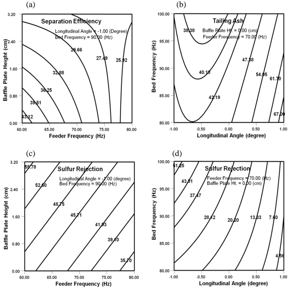
Figure 10: Simulated response surface contours generated with empirical model equations for: (a) separation efficiency, (b) tailings ash, (c) sulfur rejection with high separation efficiency as a target, and (d) sulfur rejection with high tailings ash as a target.
