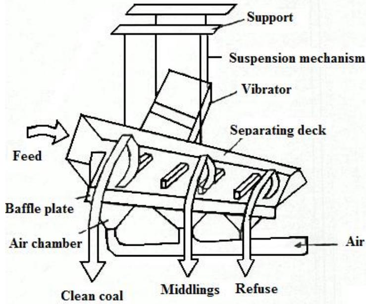
Figure 1: A schematic diagram of the FGX Dry Separator showing the different product streams (Lu et al., 2003).
