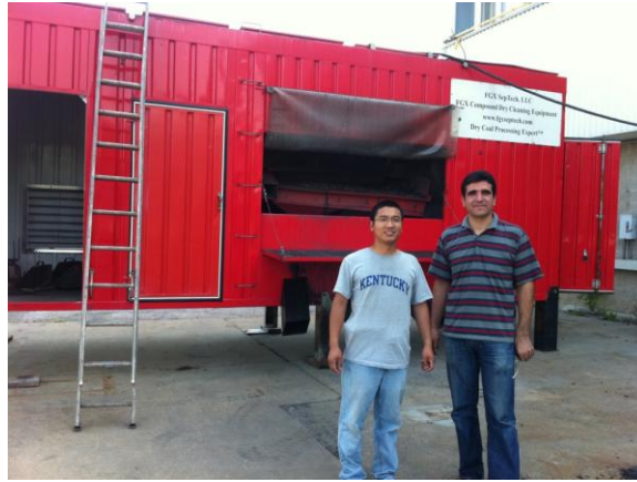
Figure 4: FGX SepTech LLC’s 10-tph FGX Dry Separator test unit.
