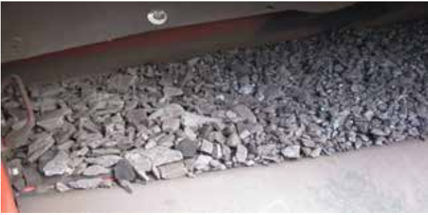
Figure 3. Distribution of clean coal and tailings on the FGX unit.
